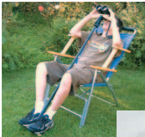
Left: Brandon Adler is seen here using the T-Pod, a photographic monopod that has been modified for binocular use. Courtesy Alan Adler.
