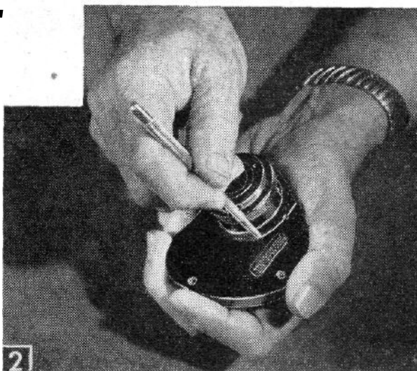
Hold the scribe against the focusing ring for a guide when scribing line.
