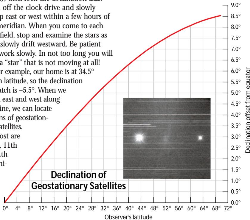
Use this graph to find the declination south or north of the celestial equator where you can spot geostationary satellites from your latitude. *Inset:* Jim Young photographed two of them, DirecTV 2 (left) and DBS-3, using a 24-inch reflector last August 16th. With the telescope's clock drive turned off, stars trailed across the field during this 1-minute exposure while the satellites remained stationary. These two are only 40 miles apart.
