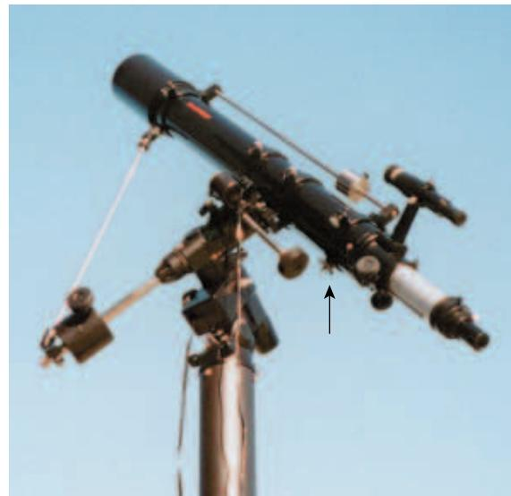
an inherently rigid structure, improved stiffness and vibration damping invariably result. In Britain such a reinforcing spar is usually referred to as a "Hargreaves strut," after the accomplished Jupiter observer, commercial telescope-maker, and past president of the British Astronomical Association, the late F. James Hargreaves.
