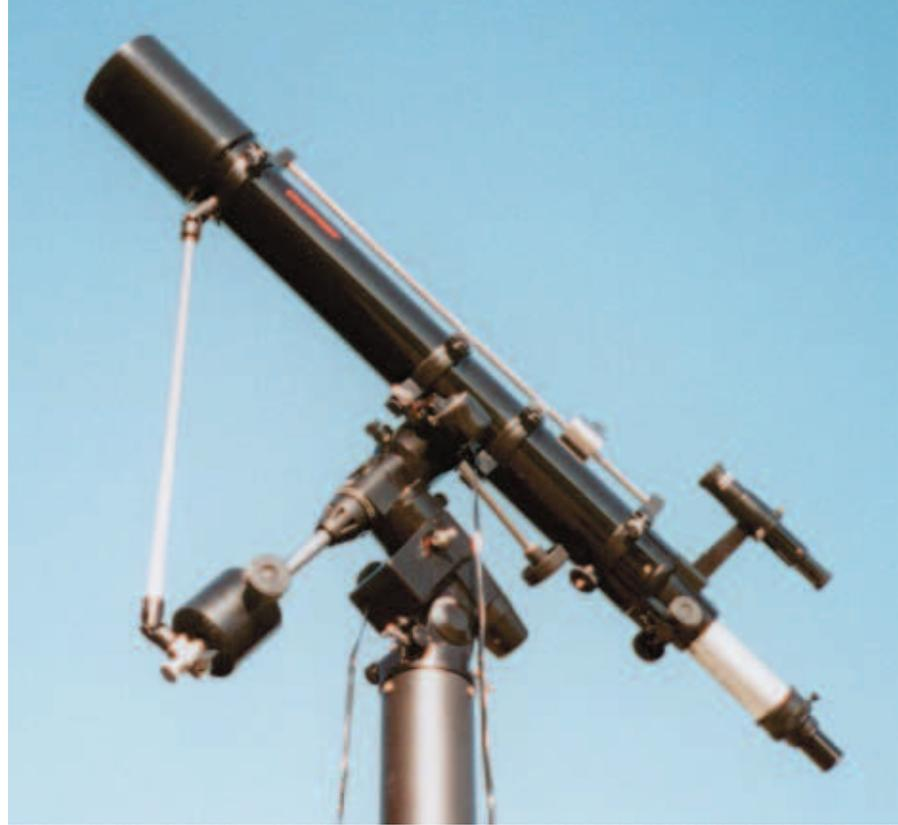
**Above:** The author's Celestron CP-102 refractor is attached to a CG-5 mount. The Hargreaves strut, which joins the objective end of the telescope with the mount's counterweight shaft, greatly improves the stability of the setup. The strut assembly is made from off-the-shelf components. All photos by the author unless otherwise specified.
