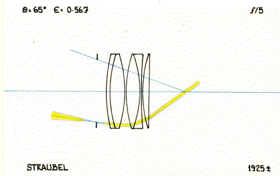
Another type of eyepiece of unknown origin is a 2-2-2 construction. This type will give an apparent field of about  $60^\circ$  at  $f/5$  and  $0.72F_e$  eye clearance. The glasses used were extra-dense flint and hard crown, barium
