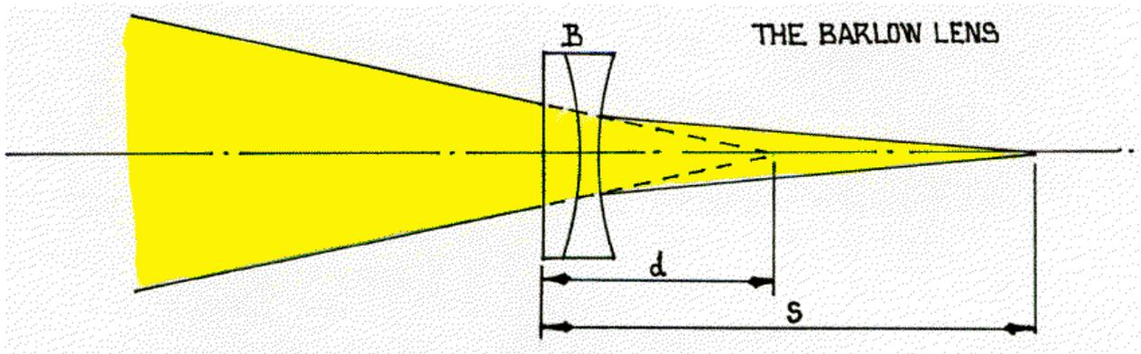
By increasing the effective focal length of the objective in this way, the focal ratio is reduced, which improves off axis performance and reduces residual chromatic and spherical aberrations owing to the smaller exit pupil.
