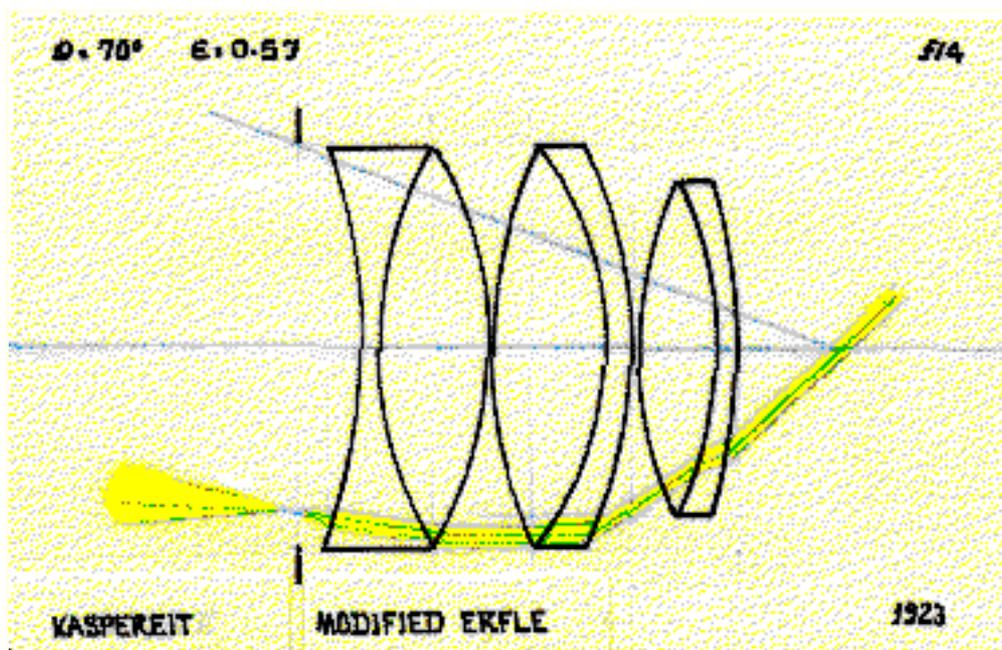
Zeiss' modification of the Plössl, and the subsequent incorporation of the field lens to widen the field, led Heinrich Erflé to design the first true wide-angle eyepiece for military use in 1917.
