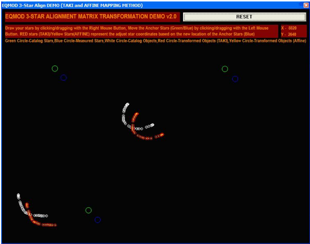
Figure 6: Here is a screen shot of the Affine Simulator showing the three stars evenly measured. If the alignment stars are accurately centered, objects even outside the triangle are accurately transformed
