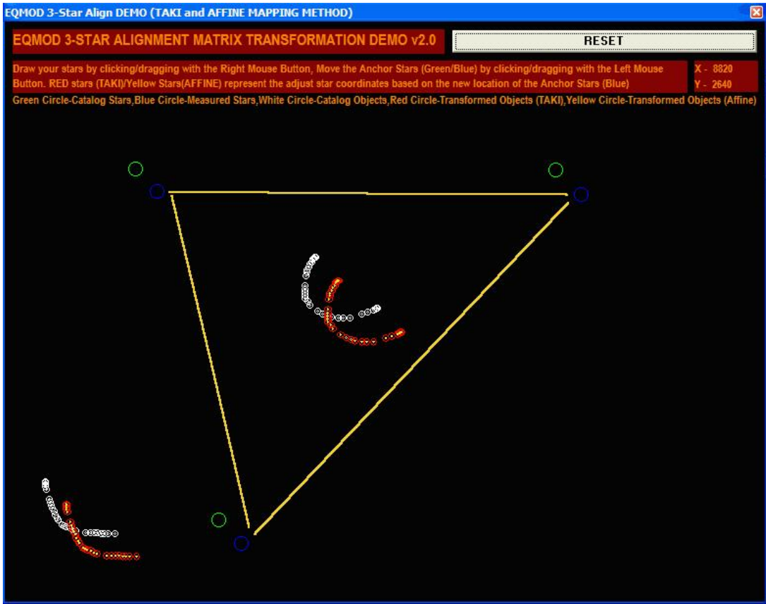
Figure 6: Here is a screen shot of the Affine Simulator showing the three stars evenly measured. If the alignment stars are accurately centered, objects even outside the triangle are accurately transformed
