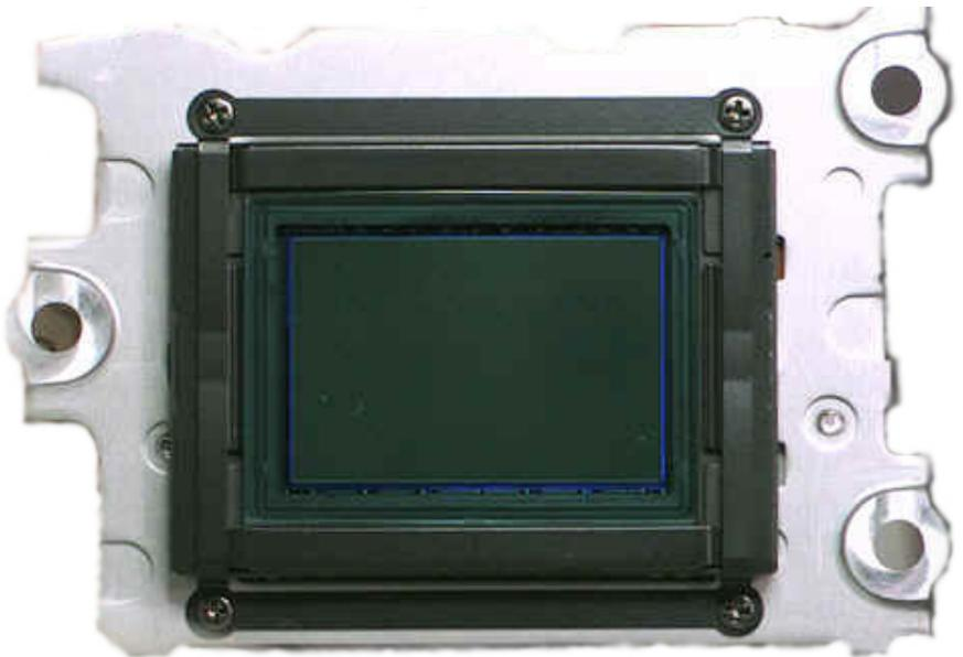
The CCD image sensors can be implemented in several different architectures. The most common are full-frame, frame-transfer and interline. The distinguishing characteristic of each of these architectures is their approach to the problem of shuttering.
