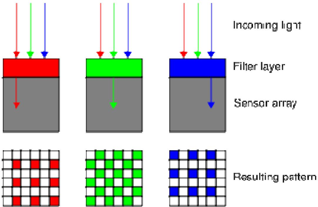
Bayer pattern on CCD sensor showing only the constituent colors passing thru.
