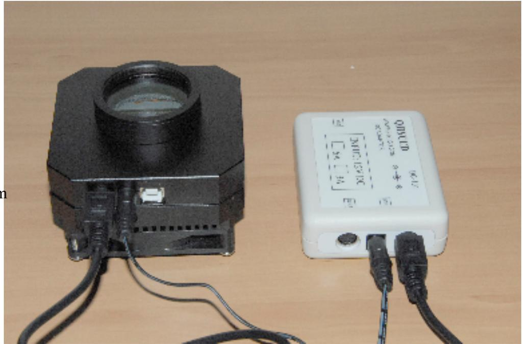
The USB socket accepts only USB2.0 interface and cables, as the camera operates at very high speeds and requires the right type of interface and cables
