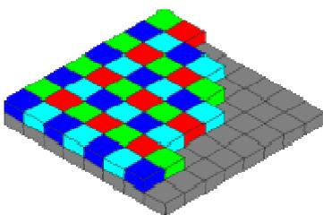
An RGBE filter on a CCD
