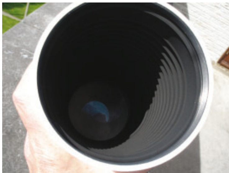
Image 7 - The baffle configuration of the optical tube are continued throughout the entire length of the dew shield.
