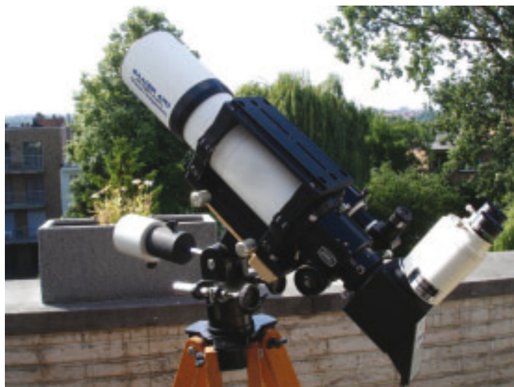
Image 4 - By unscrewing a 60-mm-long extension tube, the tube length is reduced to only 395 mm, allowing use of a binoviewer or a Herschel wedge without the need of additional transfer lenses.
