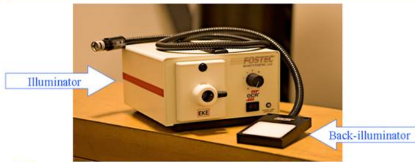
Fiber optics illuminator + Back-illuminator (Black cord from backilluminator goes into the front illuminator hole)
